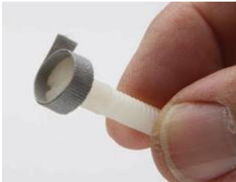
Tired of slipping off your wing bolts and damaging those nice new wings? Wrap narrow strips of masking tape several times around the head of your bolts and then give them a shot of thin CA to harden them. The resulting “fence” will prevent the screwdriver from skidding out of the slot and scarring your wing.
