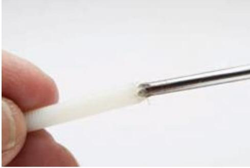
This is how to remove a broken nylon wing-mounting bolt at the field. Just heat up the end of a Phillips screwdriver (you can use a lighter or matches, or lay the bit on your car exhaust manifold), and press the screwdriver into the broken stub about  $\frac{1}{8}$  inch. The heated screwdriver will make a Phillips slot in the broken stud. Once cool, just turn and remove the broken stub.
