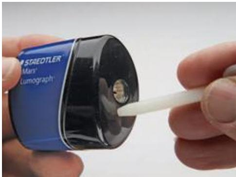
Are you having difficulty getting the nylon bolts to align with the nuts? This often happens when you try to attach the wing to the fuselage. To solve this issue, add a tapered lead to the end of the bolt using a pencil sharpener. This simple, little lead-in at the end of the bolt will improve the installation and ease of the alignment.
