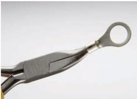
Due to the difference in diameter of standard wires and in sizes of wire from different manufacturers, it is sometimes difficult to get all the strands into the connector before crimping. Use a pair of needle-nose pliers in reverse to open up the connector's crimping end to accommodate all of the strands. When crimping, this makes for a much neater job and you won't have to trim off the wild strands.
